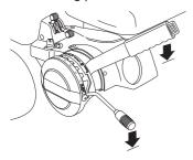
3 Push the equipment frame down and place the catch against the frame.
